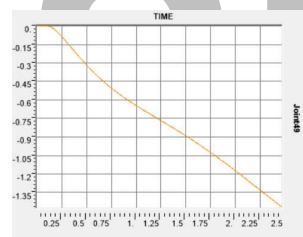
Figure 10. Deflection at column loss point in storey 1 of Figure 9
